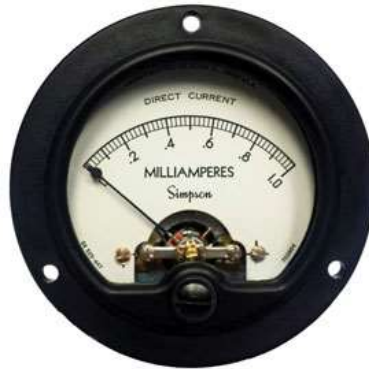
Figure 5. Common 1 mA FSD panel meters like this can be put to a lot of uses.
