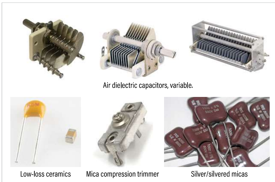
Figure 1: Various capacitors encountered in resonant circuits used in radiocommunications equipment.
