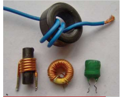
Figure 2: Various inductors that may be seen used in resonant circuits. The toroid at the top, with a few turns of heavy wire wound on it, may be used as a 'choke' to block RF current above a certain frequency.
