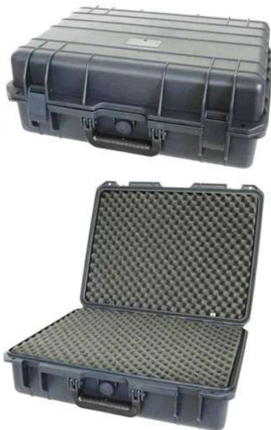
Figure 2. This clamshell style ABS "instrument case" features ribbed construction, air-tight O-ring seals, and both pluck foam and eggshell-foam inserts for equipment protection. These cases can be obtained in various sizes, ranging from 515 (w) by 200 (h) by 415 (d) mm (415 x 186 x 355 mm internal) through to 210 x 90 x 135 mm (186 x 75 x 123).
