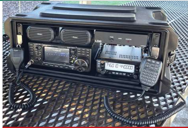
Figure 1. A Go Box station featuring two popular Icom transceivers, the IC-7300 covering 160m-6m, and the IC-2730A for 2m/70cm. The LDG model Z-100A antenna tuner at top right ensures that a variety of antennas can be accommodated. The case is a 'rack unit' type; these generally come with top and bottom covers to protect the installed equipment during transport.
