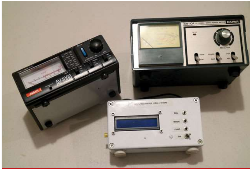
Photo 1. The two units at the top represent the sort of run-of-the-mill VSWR/Power meters that you might see in many amateurs' shacks. The box at front is a homebrew milliwatt RF power meter.
