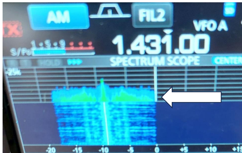
The arrow indicates the lower end of the signal band at 1.431 MHz.
