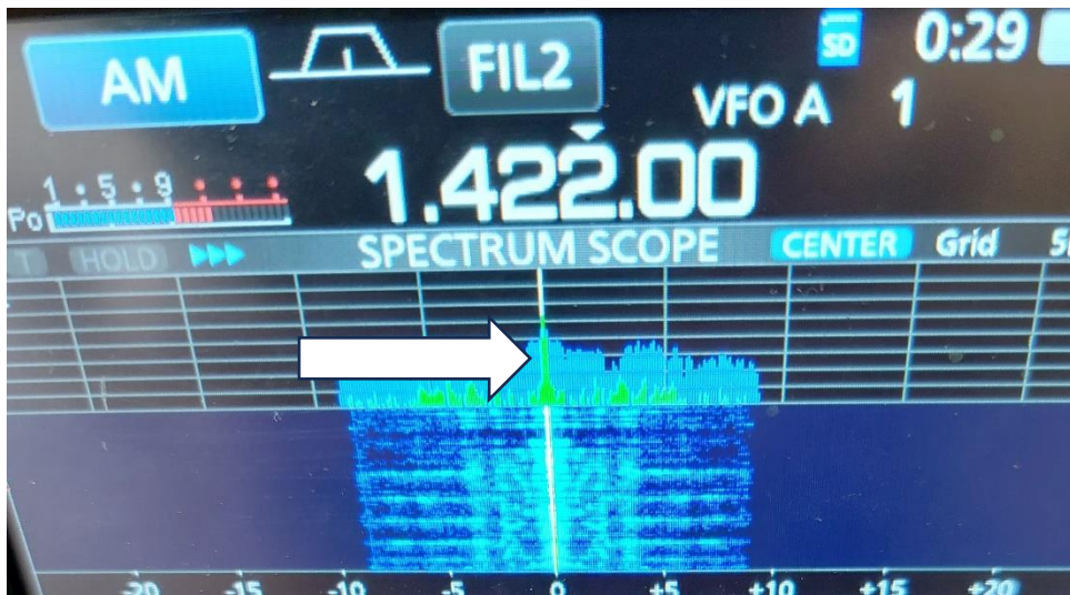
A double-sided AM signal with the carrier at 1.422 MHz.
